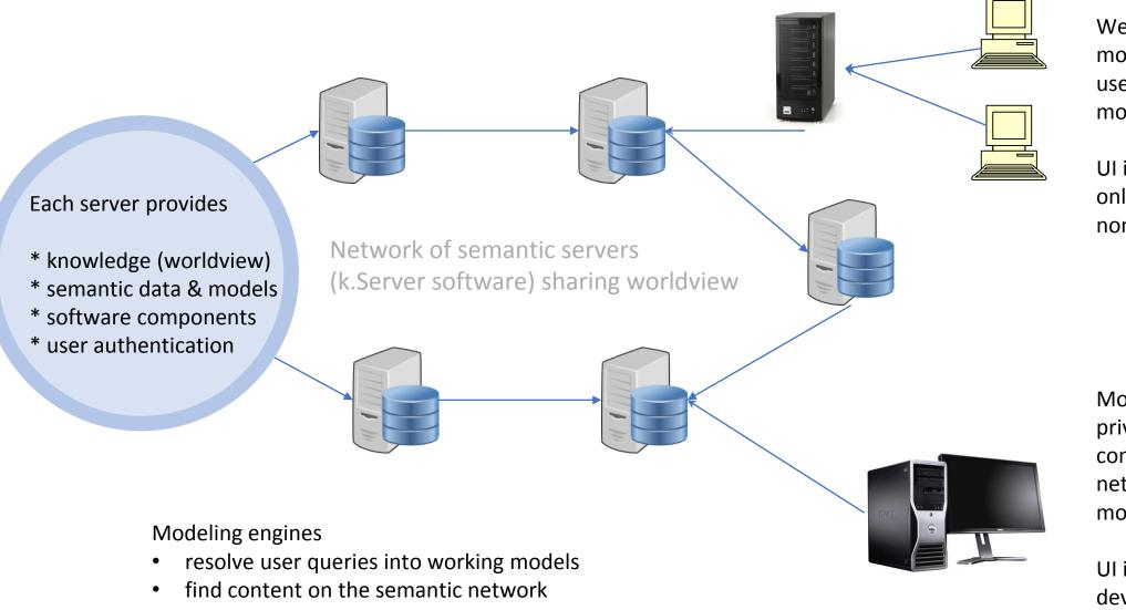
Web users connect to modeling engine and use web interface for modeling
